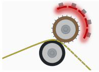
The Micro-perforation, made by melting and punching the material, is carried out thanks to needles fixed on bronze sleeves, which are mounted on the needle shaft.
