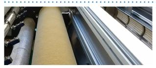
This micro-perforator is designed to punch **MICRO HOLES** in moving film using **HOT NEEDLES**. This machine has to be integrated into existing machinery such as extruders, bag machines, slitters or printing machines. The **HN150** is a **MOTORIZED**
